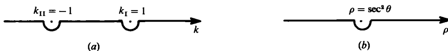
FIGURE 1. The integration path for the inversion of the Fourier transforms: (a) two-dimensional flow; (b) three-dimensional flow.
